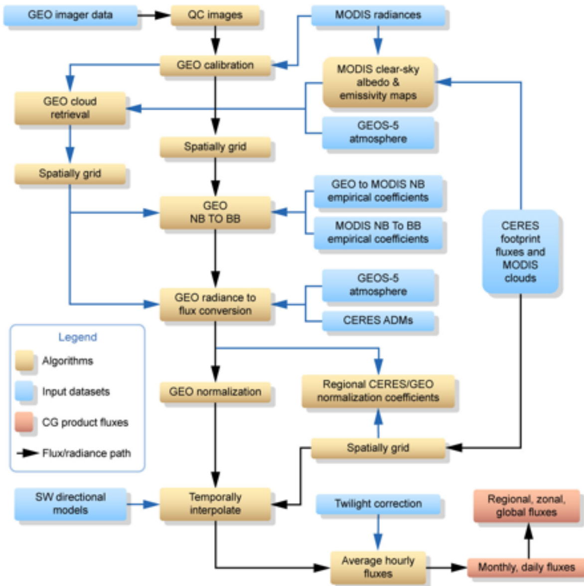
Figure B11 Flowchart of steps used to produce the CERES SYN1deg product.
