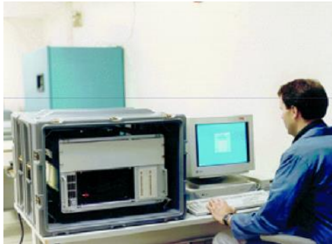
FIGURE 8.2-1 PORTABLE TEST ENVIRONMENT FOR DEVELOPMENT AND TESTING OF ELC PAYLOADS
